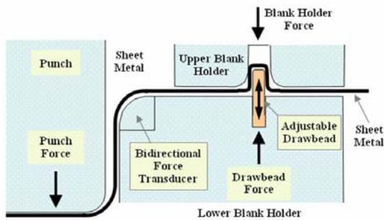
Fig.4: Active drawbead control system [25]
