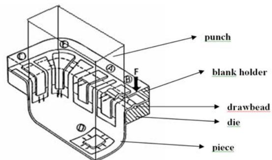
Fig.1: Complex deep drawing process
