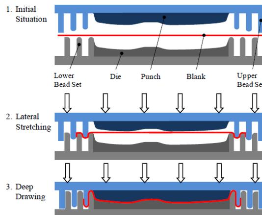
Fig. 3: Schematic view of the drawing process by SCS Tool [27]
