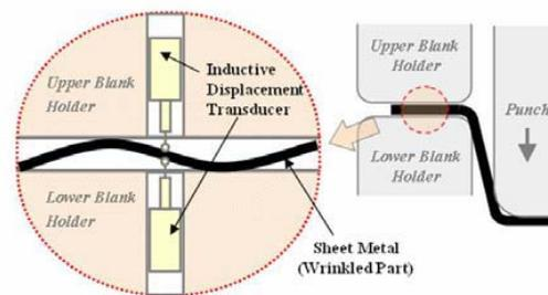
Fig. 5: Inductive displacement transducer for the measurement of the wrinkle height [32]
